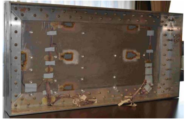
Figure 4: Instrumented aluminum plate. The strain gauges and the holes for the pressure probes can be seen. The two rows of bolts can be also recognized, which clamps the plate to the frame.
