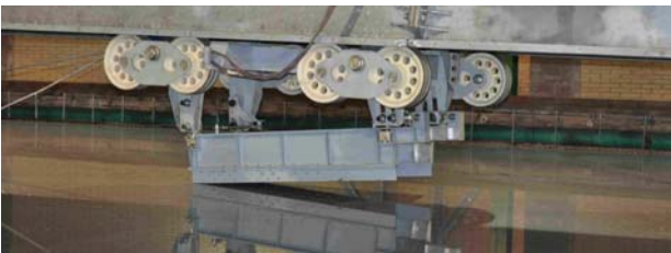
Figure 3: Picture of the trolley with model at the touch of the free surface. Note that the specimens is not installed yet.
