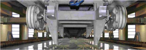
Figure 2: Picture of the main trolley which brings the model and specimens.
