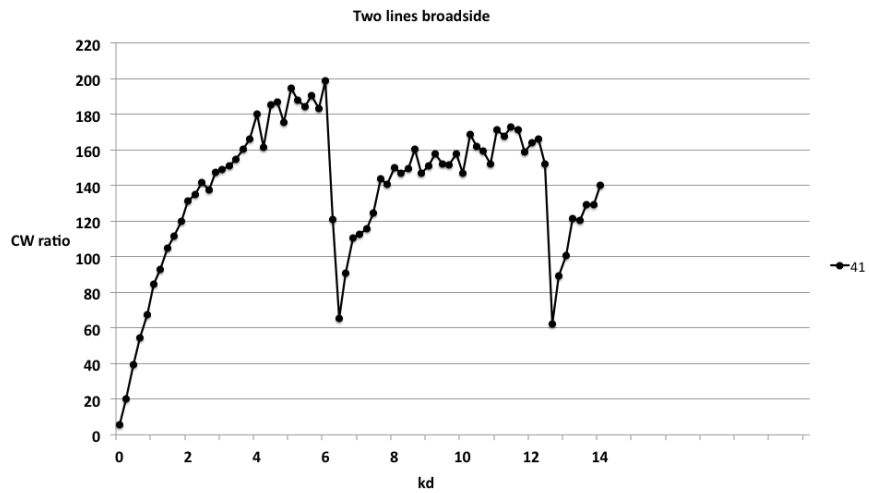
Figure 2: Capture width ratio for two parallel lines of buoys perpendicular to the wave direction, spacing d . Each line has 41 buoys.
