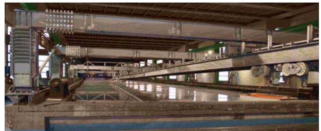
Figure 1: View of the CNR-INSEAN guided ditching facility. The guide is supported by bridges which can be varied in height in order to get the correct U/V velocity ratio. The main trolley can be also seen on the right.
